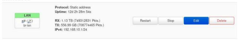
In the IPv4 address box change the IP from 192.168.10.1 to 192.168.5.1. Make a note of this change. Again, we recommend noting this on the bottom of the router alongside the log in password.
